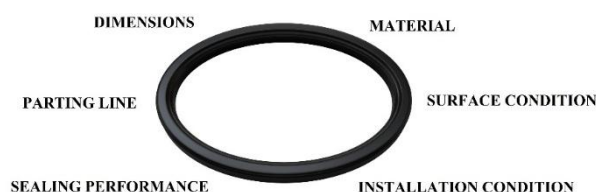
Figure 2. Main Characteristics Considered in O-Ring Inspection
